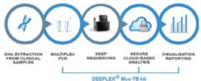
Figure 2. The Deeplex ® Myc-TB workflow. From DNA extraction from clinical or culture samples to data analysis and result visualization. The assay comes as two options: the Deeplex ® kit and the Deeplex ® service . The kit includes a single PCR master mix ready for multiplex amplification of the mycobacterial targets, positive and internal control as well as an activation code to access the Deeplex ® Web App. Service is performed at GenoScreen.
